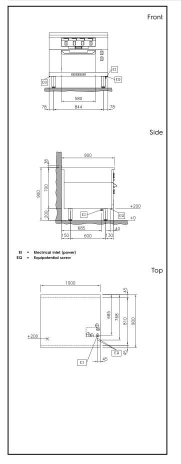
Modular Cooking Range Line thermaline 90 - 4 Zone Electric Solid Top on Oven, 1 Side, Ecotop with Backsplash, H=700 The company reserves the right to make modifications to the products without prior notice. All information correct at time of printing.
